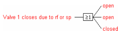
Illustration: Minimal cut to the fault tree “Valve 1 closes due to rf or sp”
